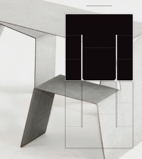
The basic shape is exactly half the size of a standard 3 x 1.5-meter aluminium sheet. Apart from the saw cuts and minimal rounding off, material wastage is nil.
